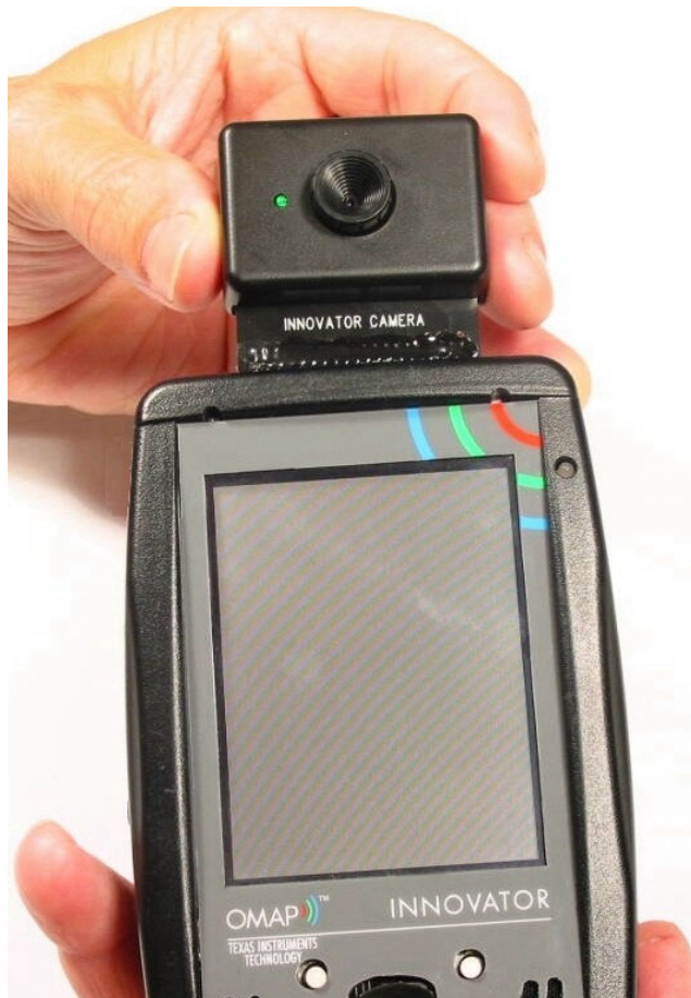
Figure 38. Camera Installation, Facing Forward
