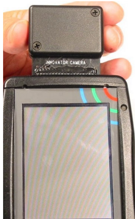
Figure 39. Camera Installation, Facing Backward
