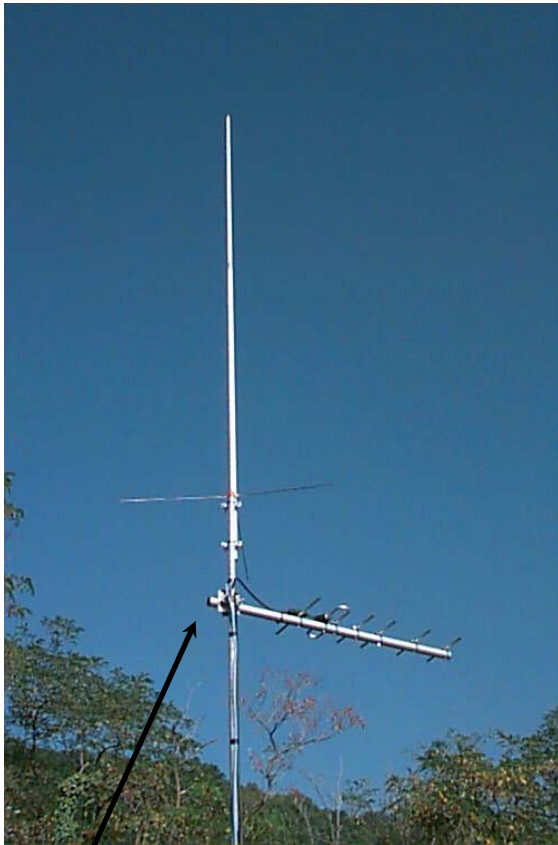
■ Omni Directional Antenna
