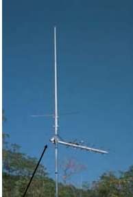
■ Omni Directional Antenna
