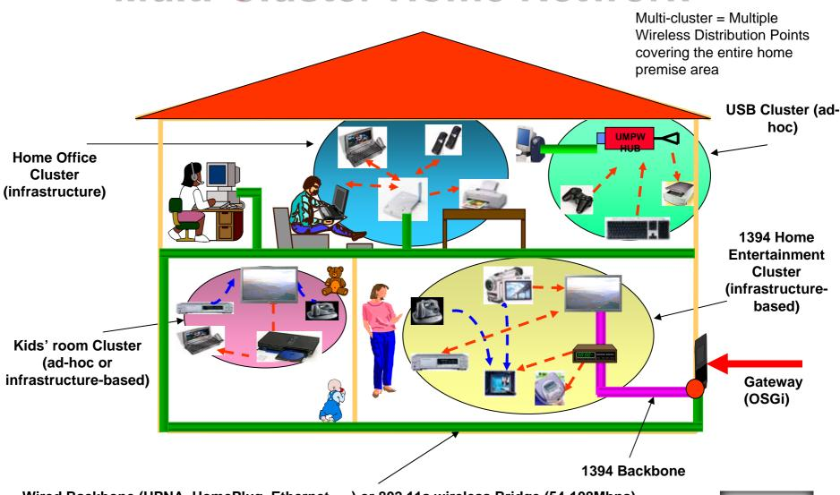
Wired Backbone (HPNA, HomePlug, Ethernet, ...) or 802.11a wireless Bridge (54-108Mbps) Wireless & Multimedia Network Laboratory™
