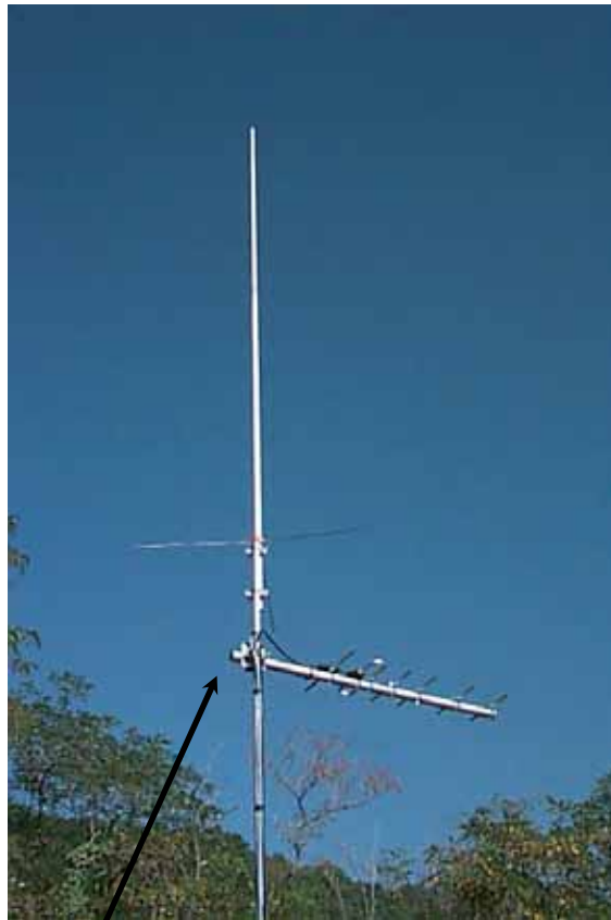
■ Omni Directional Antenna
